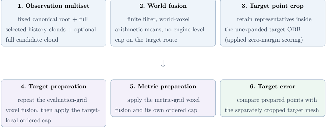
Figure 4: Result-affecting preparation order for both the current and candidate-appended target states, read 1 \rightarrow 2 \rightarrow 3 , then 4 \rightarrow 5 \rightarrow 6 . Configurations may make two voxel stages numerically redundant, but their distinct caps and declared grids remain separate protocol stages.
